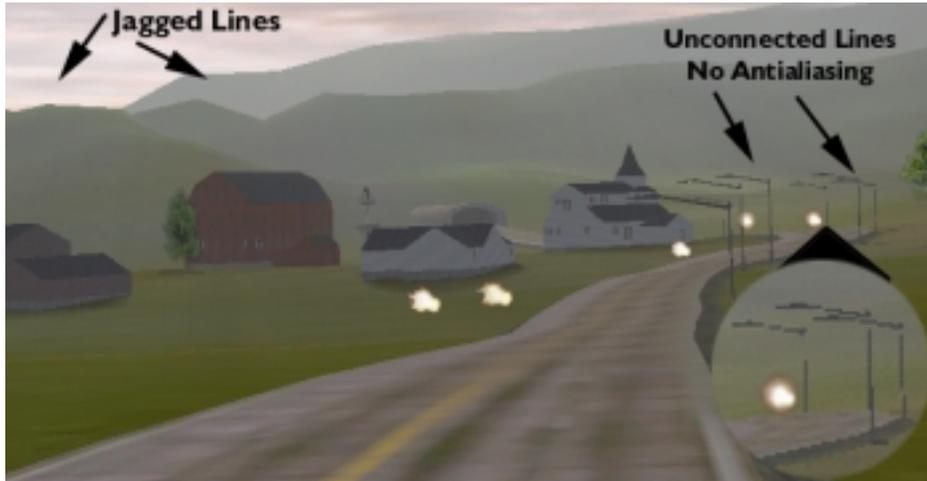
Figure 3 (top): The aliasing in the image to the left shows as both jagged, or stair-stepping, lines and as broken lines. The jagged lines are very noticeable on the edges of the mountains in the upper left area of the scene. The broken lines show in the light poles in the lower right.
